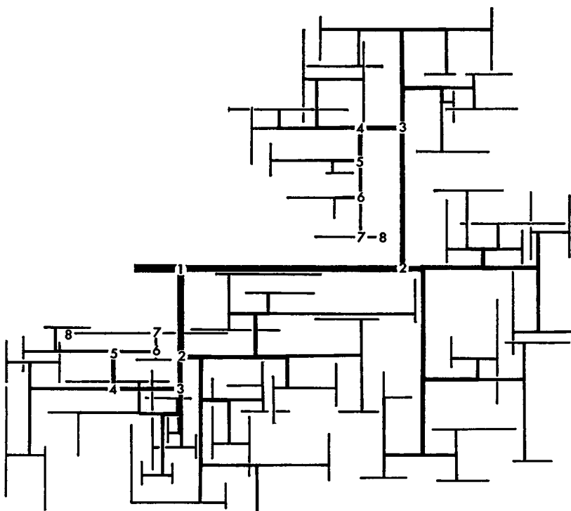
FIGURE 1 The assembly of branching tubes used in the calculation; lengths of branches to scale, diameters not to scale. The numbers indicate the short (at left and below) and long (at right and above) pathways over which transmission was studied.
